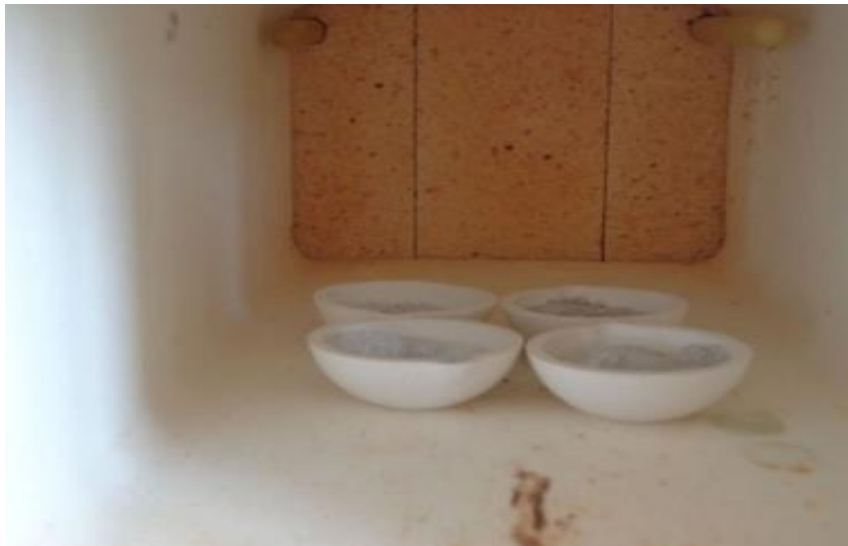
Illustration (3.1). Powder calcination.
