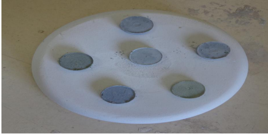
Illustration (3.2). The results of the pressing process samples .
